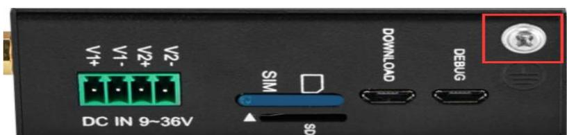
Before connecting the device, please do equipment grounding with grounding screw to prevent electromagnetic interference
