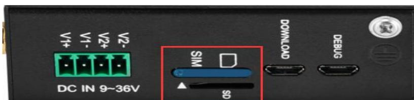
Make sure device is powered off before inserting or removing SIM card. Insert SIM card Picking PIN into the hole with tiny force to eject out the card tray.
